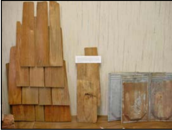
The photo at left shows some of the shingles that were found in the attic of the house when restoration began. The shingles to the far left are hand split cypress shingles that had never been used. The two shingles in the center, also hand split cypress, show signs of use and were probably part of the original roof. The cypress shingles were replaced by the galvanized stamped metal shingles.
