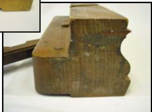
These photos show a nineteenth century molding plane that would have been used by craftsmen of that period to produce decorative moldings. The photo at right shows the molding profile of this plane. This molding plane is a part of the Sam Strauss Collection of Historic Woodworking Tools, a collection belonging to the Arkansas State University Museum in Jonesboro, Arkansas.
