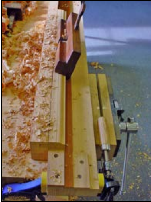
Early American window muntins were made by skilled craftsmen using hand held molding planes. This photo shows a demonstration of decorative molding being cut on the interior side of a window muntin using a sash molding plane. This molding profile is called a sash ovolo.
